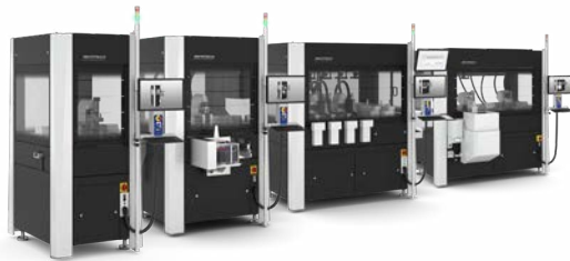
High Speed Production Cells; 3m/s axis speeds and form factors ranging from 900 mm up to 2,000 mm
